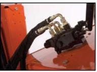
The four-position valve easily controls the hydraulic feed roller
